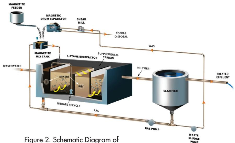
Figure 2. Schematic Diagram of BioMag Process (from Siemens)
