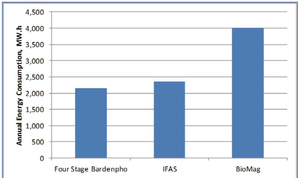
Figure 5. Comparison of Energy Requirement
