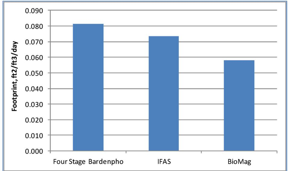
Figure 4. Comparison of Process Footprint (Required Area/Flow to be Treated)
